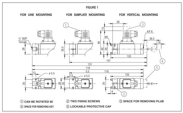
Please refer above figure. HM model pressure switches can be mounted in any direction. There are three different mounting options.
